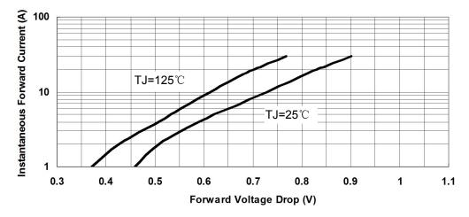
Fig.3-Typical Instantaneous Forward Voltage Characteristics
